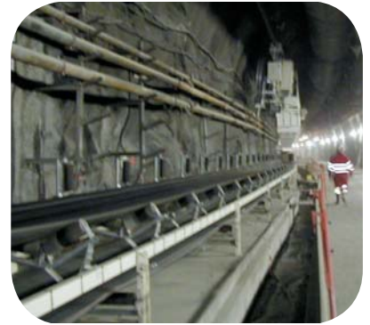
Transporteur au sol Belt conveyor on the ground
